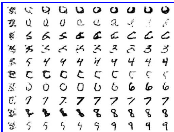
Figure 9: Each row shows 10 samples from the generative model with a particular label clamped on. The top-level associative memory is initialized by an up-pass from a random binary image in which each pixel is on with a probability of 0.5. The first column shows the results of a down-pass from this initial high-level state. Subsequent columns are produced by 20 iterations of alternating Gibbs sampling in the associative memory.
